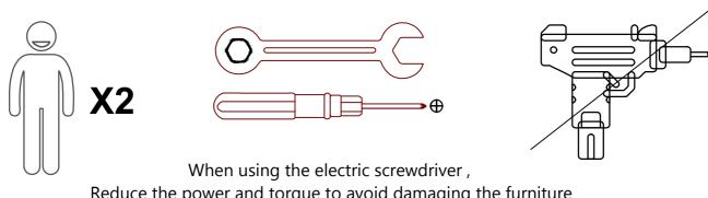
Reduce the power and torque to avoid damaging the furniture
