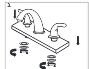
STEP 3. Place the handle bodies through the left holes. Re-assemble the parts and screw with lock nut.
