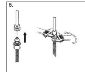
STEP 4. Connect handle assembly to the faucet body with water supply hose. Push supply hose adapter with hose coupling until you hear a "click".
