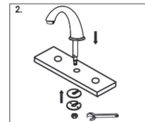
STEP 2. Place the spout in the center hole of the sink. Secure faucet as shown above.
