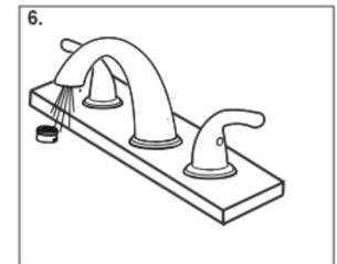
STEP 6. After installing faucet, remove aerator and turn on water to remove any left over debris. Re-assemble aerator.
