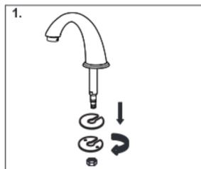
STEP 1. Remove assembled parts from the faucet body.
