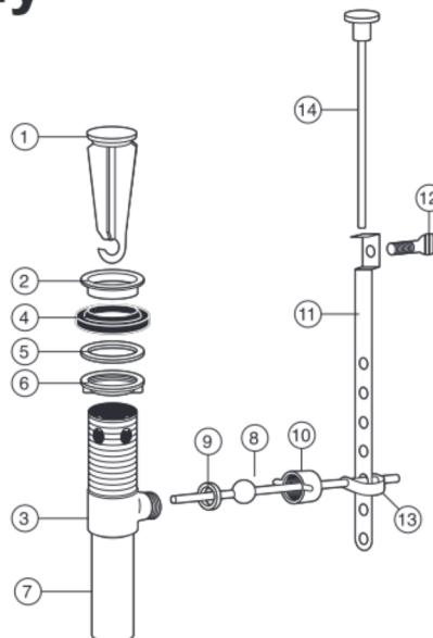
9. Adjust the height of the lift rod by loosening up the thumb screw and resetting it tightly.
