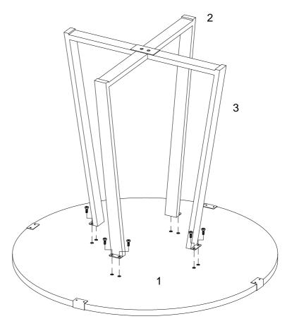
Attach part (2, 3) to part (1) using bolt (A) with hex key (C).
