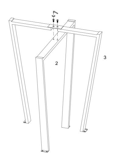
Attach part (3) to part (2) using bolt (B) with hex key (C).
