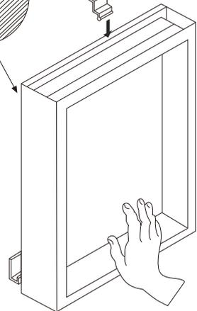
Insert top mounting bracket into the top of the cabinet.
