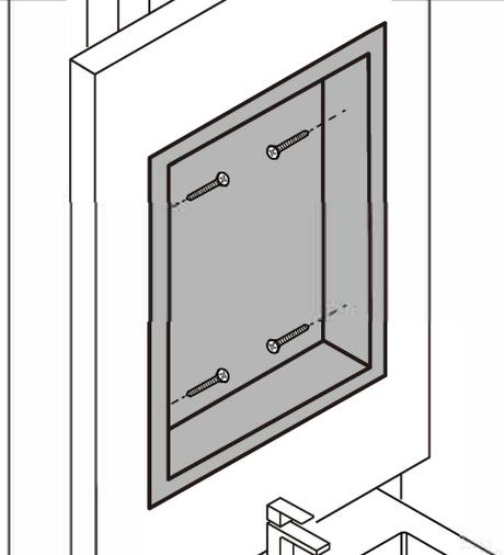
Affix using hardware screws into the studs.
