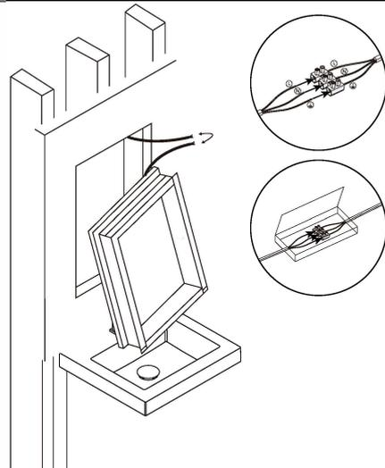
Connect electrical wires before inserting the cabinet into the opening.
