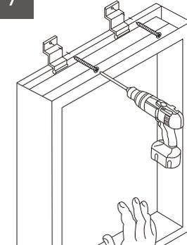
**!** Top mounting brackets must be attached to furring strip/channel or wall studs.
