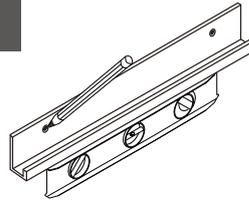
**!** Bottom mounting brackets must be attached to furring strip/channel or wall studs.
