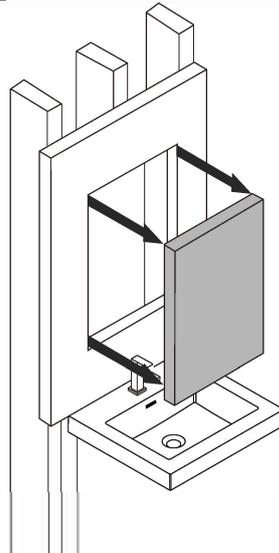
Cut the marked perimeter with suitable tool.
