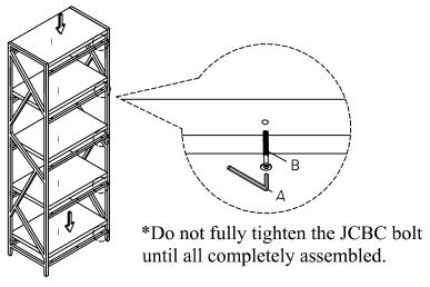
Attach back rail (5,6,7) to side rail (2,3), JCBC screw (B), tighten by using allen-key (A). Secure with bracket-tip restraint (C).
