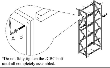
Attach fixed shelf (1) to metal rail (4), JCBC screw (B), tighten by using allen-key (A).
