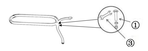
Loosely attach the Central Support Ring(C) to Table Legs(B) using Washers, Spring Washers, and Hex Bolts(①), with the Spanner(③).
