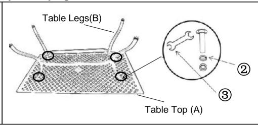
Lay the Table Top(A), top facedown onto a flat, soft, clean surface. Attach the Table Legs(B) to the Table Top(A) using Washers, Spring Washers, and Hex Bolts(②) with the Spanner(③).
