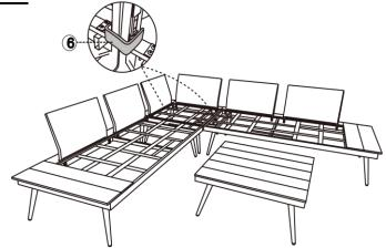
Use the Connecting Piece(6) to connect the chairs together as shown in the picture.
