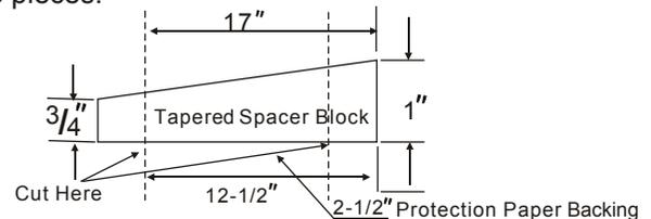
4. The 2<sup>1</sup>/<sub>2</sub>" section is placed in front of the rib on base with the tapered end facing the back of the sleeve. Cut the remaining portion to 12<sup>1</sup>/<sub>2</sub>" and place behind the rib again, sloping toward the rear of the sleeve. This helps to induce a rearward slope on the unit.
