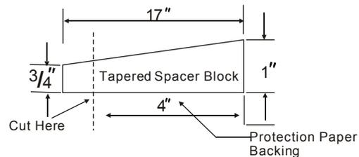
4. The 4" section is placed in front of the rib on base with the tapered end facing the back of the sleeve. The remaining portion behind the rib again is sloping toward the rear of the sleeve. This helps induce a rearward slope on the unit.
