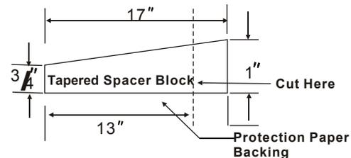
3. Install 13" section as shown with the tapered end 1/2" from the back of the sleeve. This helps induce a rearward slope on the unit.
