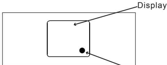
The display shows the set temperature in “°C” or “°F” and the Auto-timer settings. While on “Fan” only mode, it shows the room temperature.
