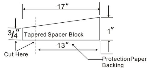
3. Install 13" section to the floor of the sleeve as shown. This helps induce a rearward slope on the unit.
