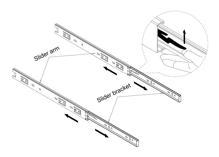
· Separate the slider bracket from the slider arm as per diagram.
