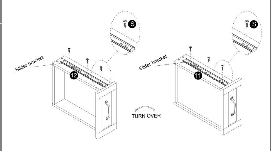
· Attach slider brackets to panels (11,12) with screws (S) correctly.
