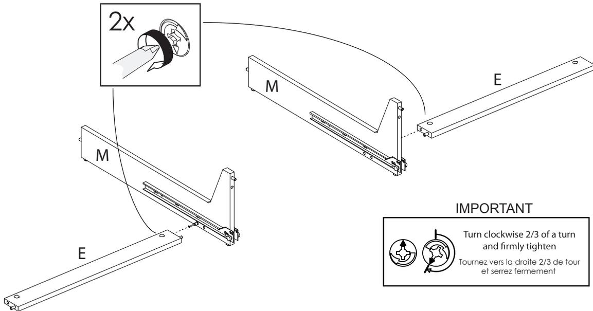
**7** Use the Allen key # 2300 and 4 screws # 0111 to fasten the panel R to both pre-assembled panels E-M
