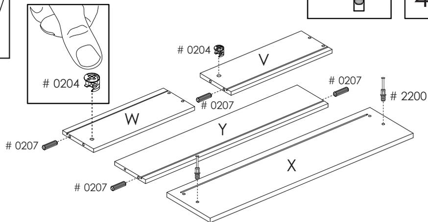
**15** Fasten the panels V and W to the drawer front X and tighten the 2 cam locks # 0204
