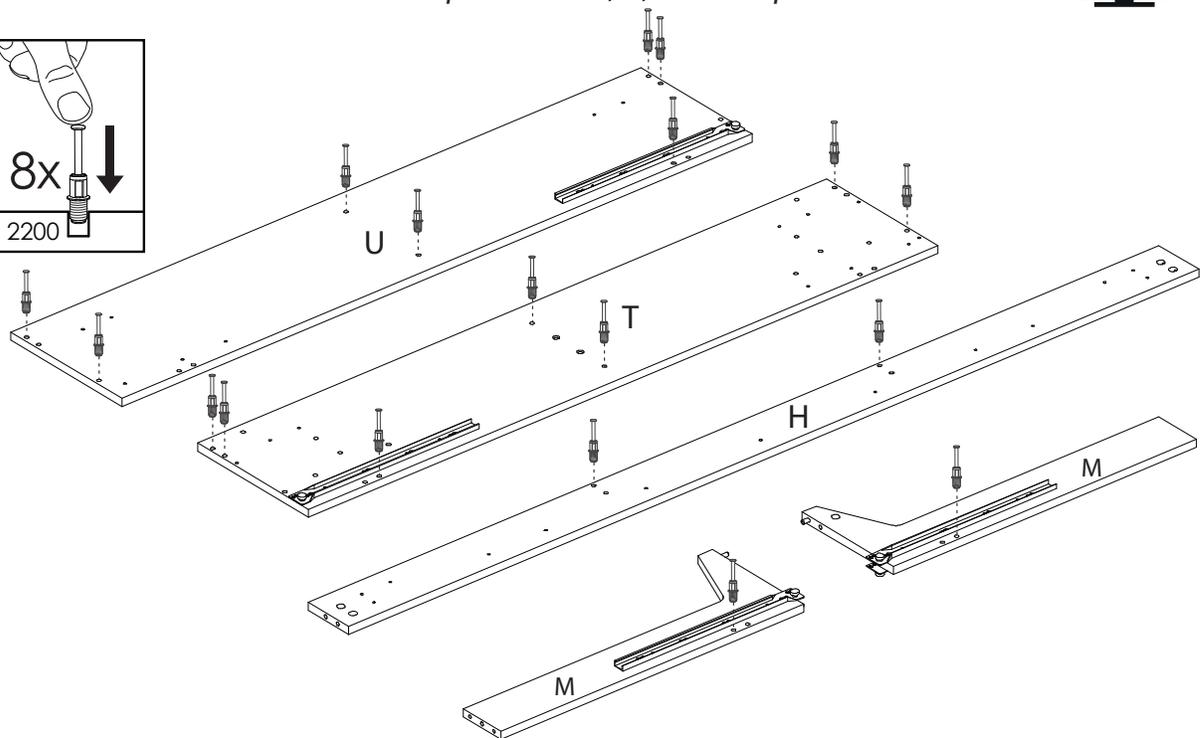
**4** Use a hammer to fasten the 8 tack glides # 1119 to the panels M, T and U
