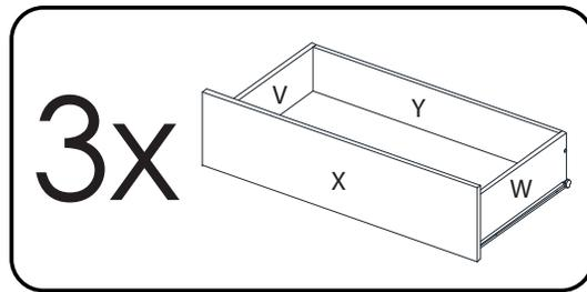
**14** Install 2 small cam locks # 0204 on panels V and W. Install 2 push bolts # 2200 on the drawer front X. Install 4 wood dowels # 0207 on panels V, W and Y
