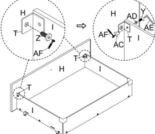
Insert the Bolt (AA) and Washer (AD) to the back of Drawer Front Board (H), turn the Ratchet Tool (AF) to tighten them.
