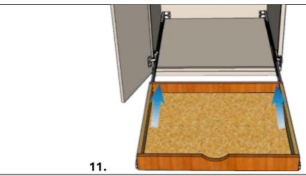
**11.** Finally, connect the sliding track and insert the drawer all the way in. You will hear the plastic latch locking into place. It is recommended to pull it out two to three times to ensure it slides smoothly. If necessary, adjust and tighten the screws on the rear bracket.
