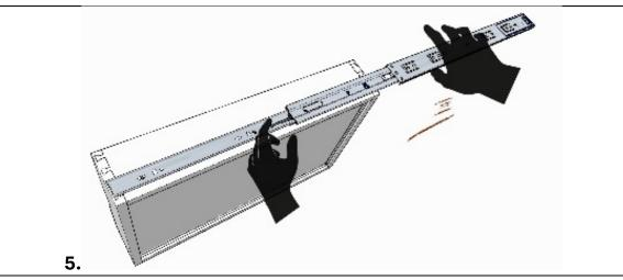
**5**. Hold the black plastic latch and forcefully pull the second and third parts of the slide rail to separate them.
