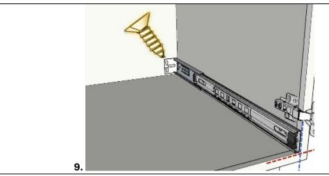
**9.** Adjust the rear bracket to the appropriate position and screw in the screws. Be careful not to tighten the screws too much, as the position may need to be slightly adjusted. Use a level to ensure the track is horizontal.
