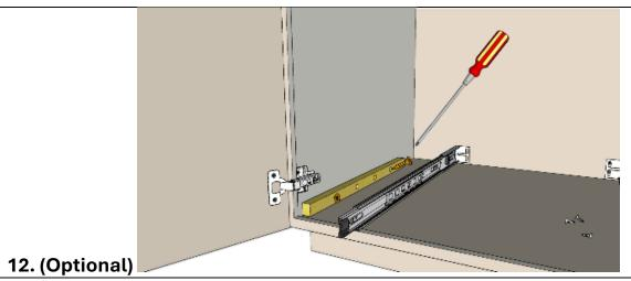
12. If necessary, wooden spacers can be used between the track and the cabinet. (Optional)
