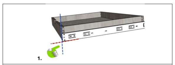
**1.** Place the drawer slide naturally on the side panel of the drawer, aligning the front of the slide with the front of the drawer and the bottom of the slide with the bottom of the drawer
