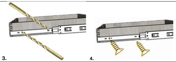
**3.& 4** Before driving the screws into the drawer, first drill a pilot hole using a 1/16" drill bit. This step is crucial.
