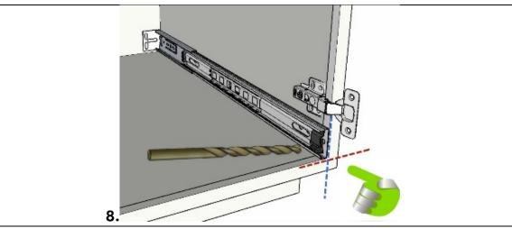
**7. & 8** Place the rear bracket on the separate slide rail. Insert it on one side of the cabinet, ensuring the front of the rail is flush with the outer frame of the cabinet and does not extend beyond the cabinet's outer edge. use a 1/16-inch drill bit to drill a pilot hole in the cabinet and then use the screws.
