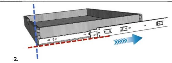
**2.** Continue to keep them aligned and slide the second and third sections of the drawer slides horizontally along the bottom of the drawer, exposing the first section of the slides.
