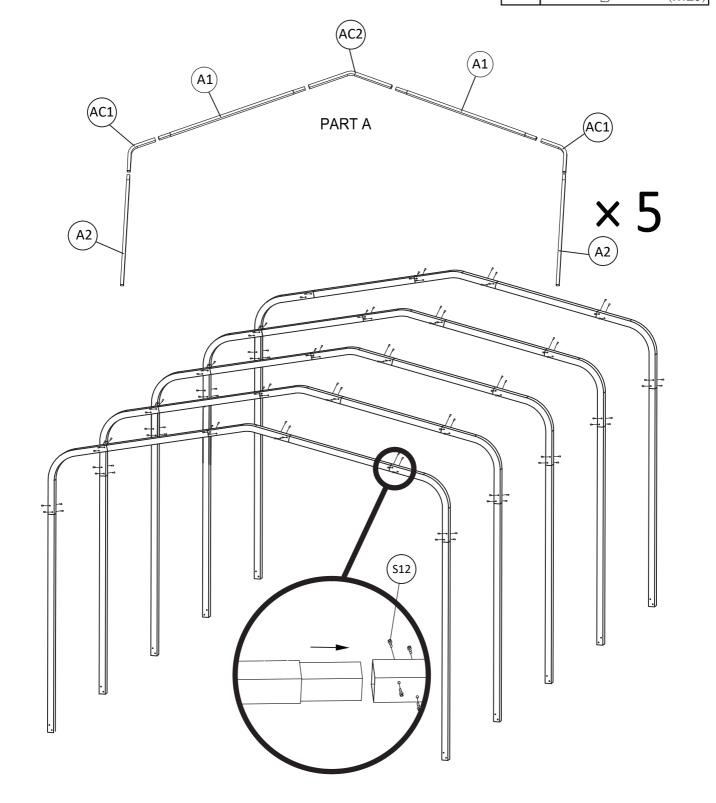
Place the two bases parallel to each other and measure the left-right distance at the front and back ends. Maintain a distance of 11.97ft between the outer edges of the bases.
