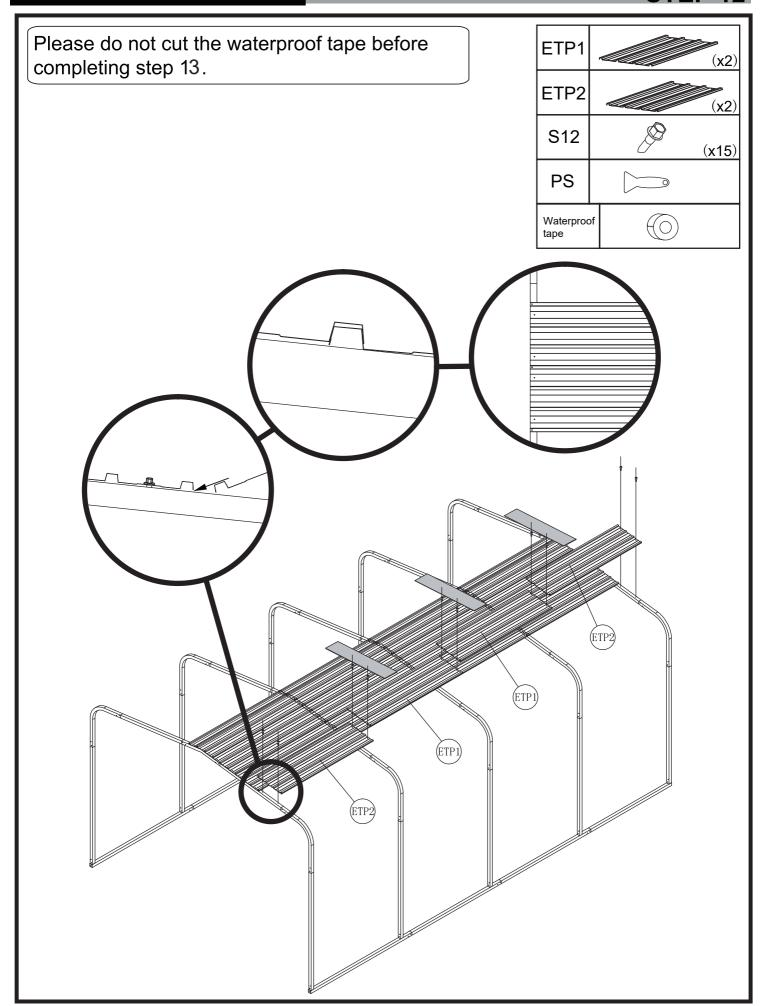
After installing the top panels, proceed to install ETP1 the side panels (Side panels can do not require (x4)waterproof tape to keep them looking nice). ETP2 Please do not cut the waterproof tape before (x4) completing step 13. S12 (x30)PS Waterproof (0)tape
