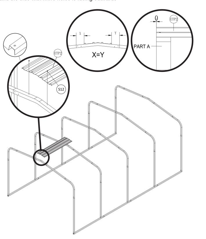
Then install the panel at the rear central position, ensuring each subsequent panel overlaps the previous one. Drill screws first, then apply a strip of waterproof tape. Ensure the edges of the panels are flush with the edges of the brackets. Please do not cut the waterproof tape before completing step 13.
