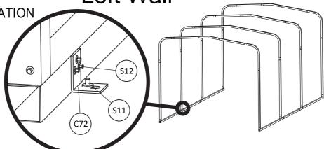
TIPS: After installing the top, measure the distance of the base, adjust it to the correct value, and fix the base.
