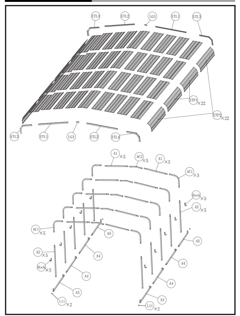
Drill self-drilling screws into the pre-drilled hole points according to the positions (installing screws diagonally increases the bracket's resistance to bending). Use your foot to hold down the steel pipe during installation to prevent sliding when drilling.
