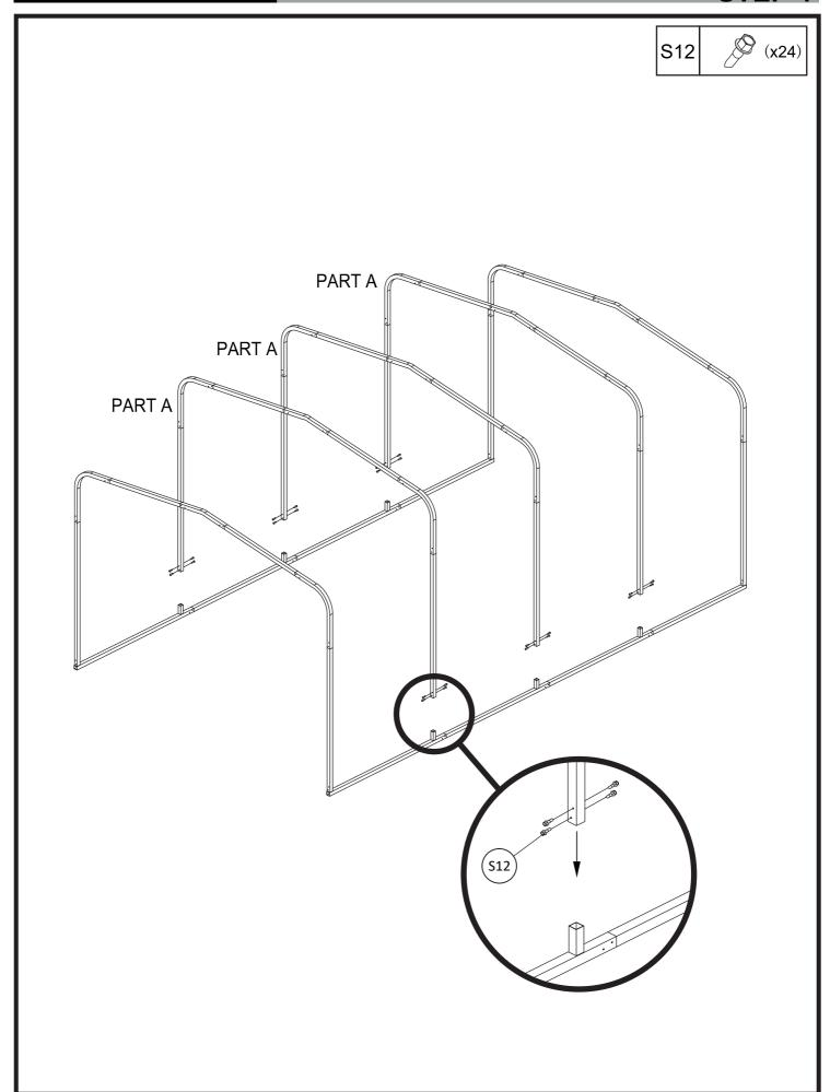
After installing all the brackets, double-check the dimensions of the base, adjust them to the specified size, and then fix the base.
