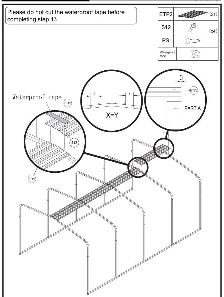
Once the central panels are installed, proceed to install the remaining panels on both sides. The outer panels should fit under the inner panels, and each subsequent panel should overlap the previous one.
