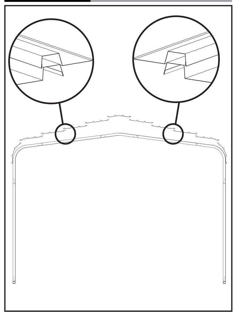
Start by installing the front panel at the central position, ensuring it is centered with a ruler.
