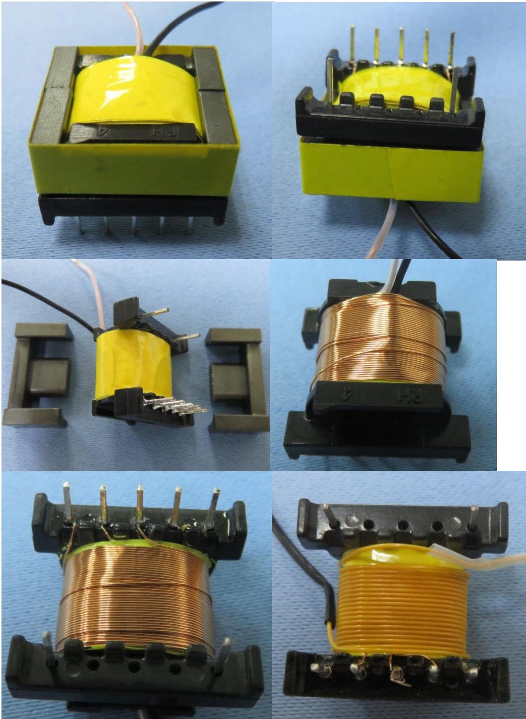
Photo 17 - Transformer view of RYJ-23 series, also represent models RYJ-18 series and RYJ-26 series
