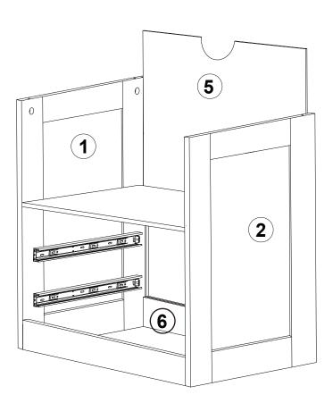
Insert Board 5 into the grooves on Board 1, 2 and 6.
