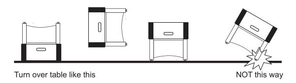
Table may become damaged if it is placed to the floor in an angle.
