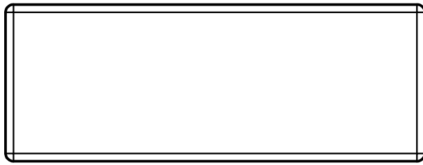
(2) J6 - SUPPORT BLOCK - W4L07589 1"x2 3/8"x6 1/4" (24x60x160)
