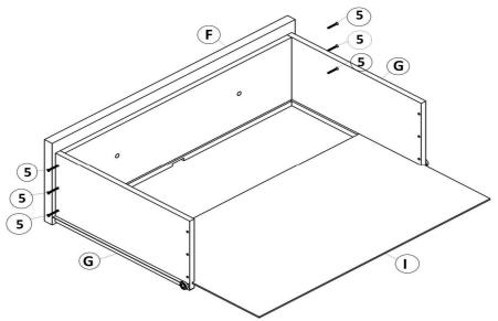
Attach drawer back (H) to drawer sides (G) with screws (5) as shown below. Tighten with a screwdriver.
