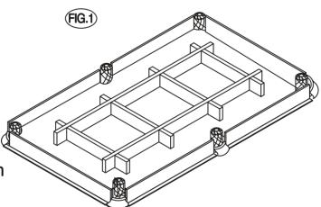
Step 2- Secure the 22 pieces of iron (#9) to the baffles (#2 and #3) with screws (#8) as shown.
