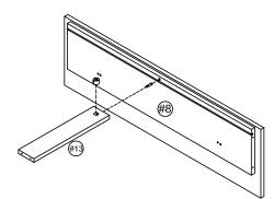
(D) x 1 cam bolt 27mm (E) x 1 cam lock Ø13.5x10.5mm
