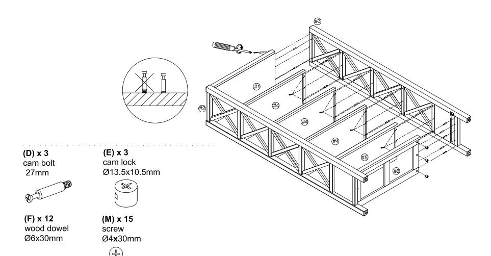
1. Screw-in cam bolts must be screwed down flush.
