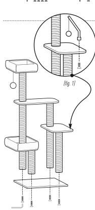
Add the assembled unit to the base. Use the long screws for the base. Tighten securely.
