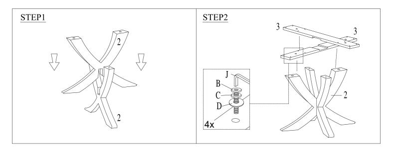
On a flat surface, place Table Legs (2) perpendicular to each other mating the half-lap joint as shown.
