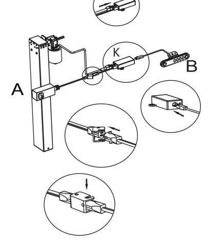
Stand the desk up, press the outlet box firmly into the desktop and use the wire clips to tide up wires
