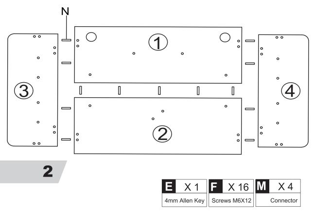
Note: The horizontal bar on the connector should be perpendicular to the seam of table panel slice
