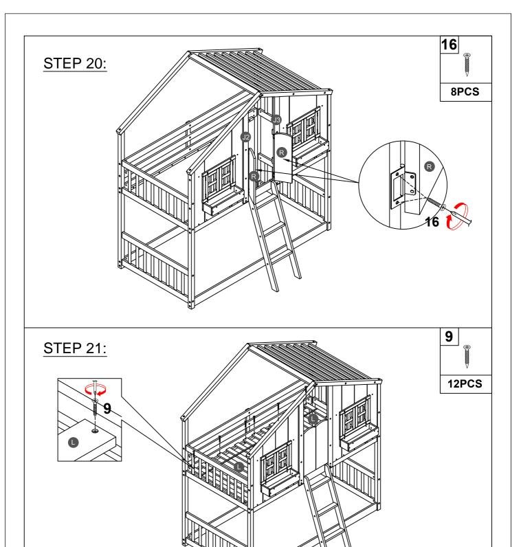
Note: Do not lock the screws of the bed slats to the outermost edge of the bed slats, you need to leave a certain space at the edges, otherwise it will cause the board to break. Do not lock the bed slats on the edge of the wood, please hold firmly before screwing, hold it in place with one hand, then lock the screw.
