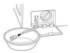
**4** Remove the pump filter.
