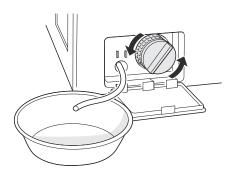
**5** Clean the pump filter and opening.
