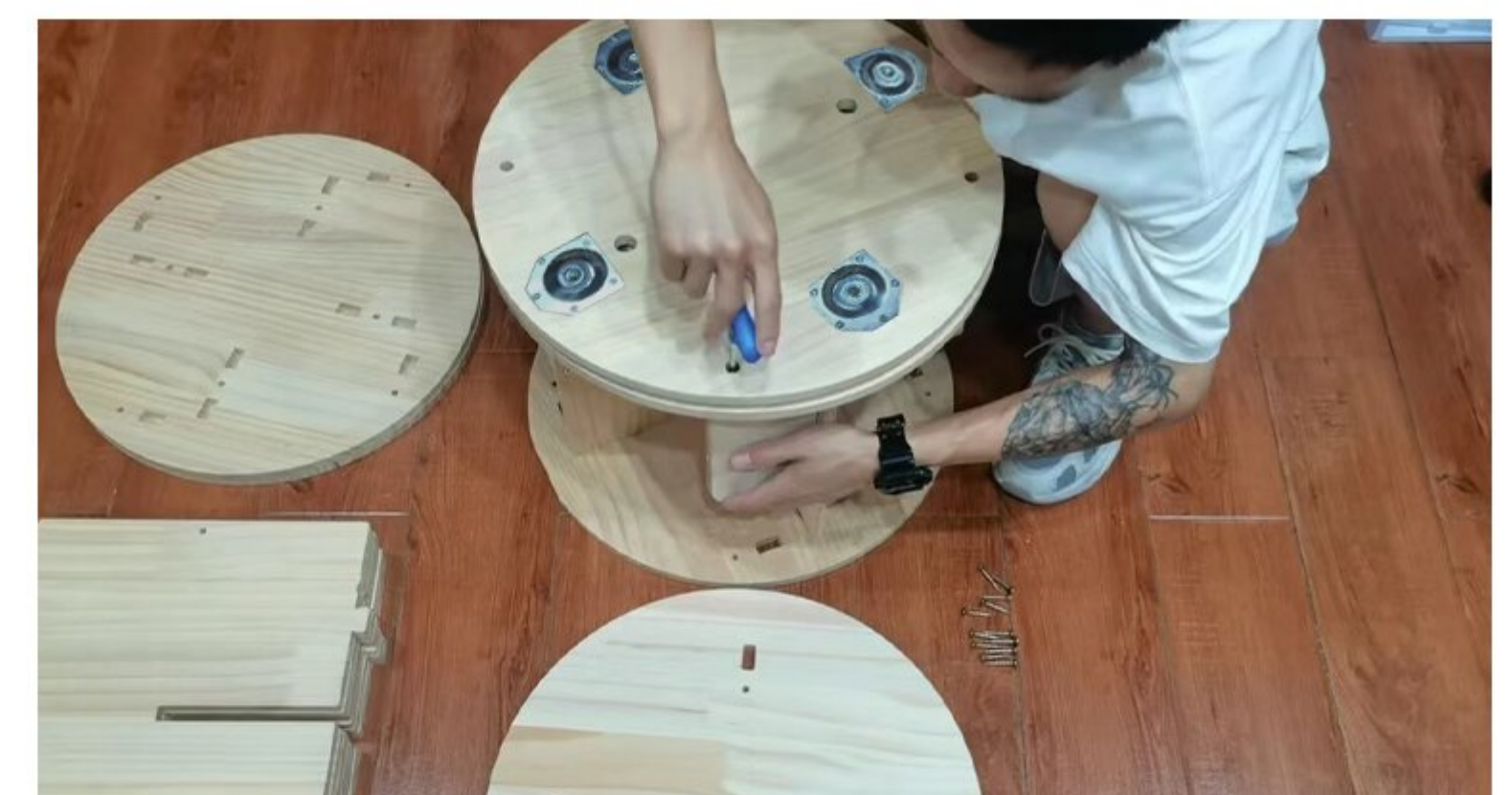
6.SCREW ON THE BOTTOM OF E-PLATE
