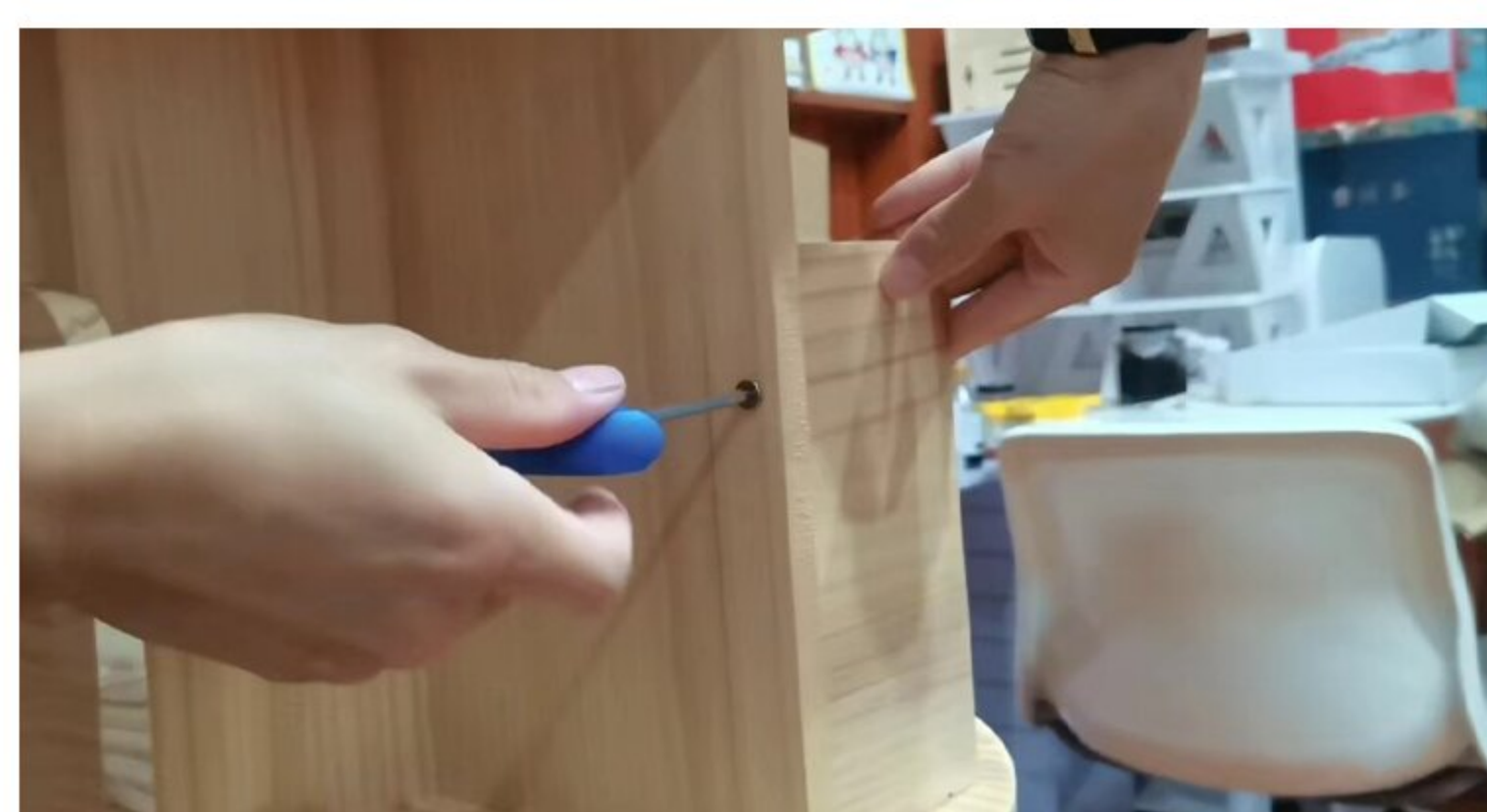
10.SCREW ON THE SIDE OF EACH E-PLATE
