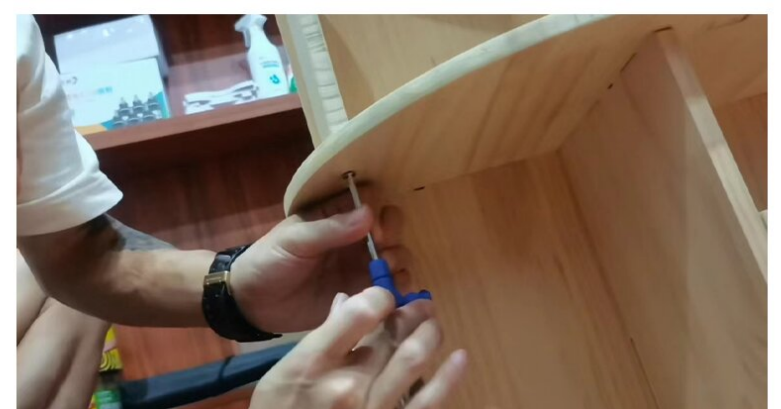
11.SCREW ON THE BOTTOM OF EACH E-PLATE FOR SECONDARY FIXATION
