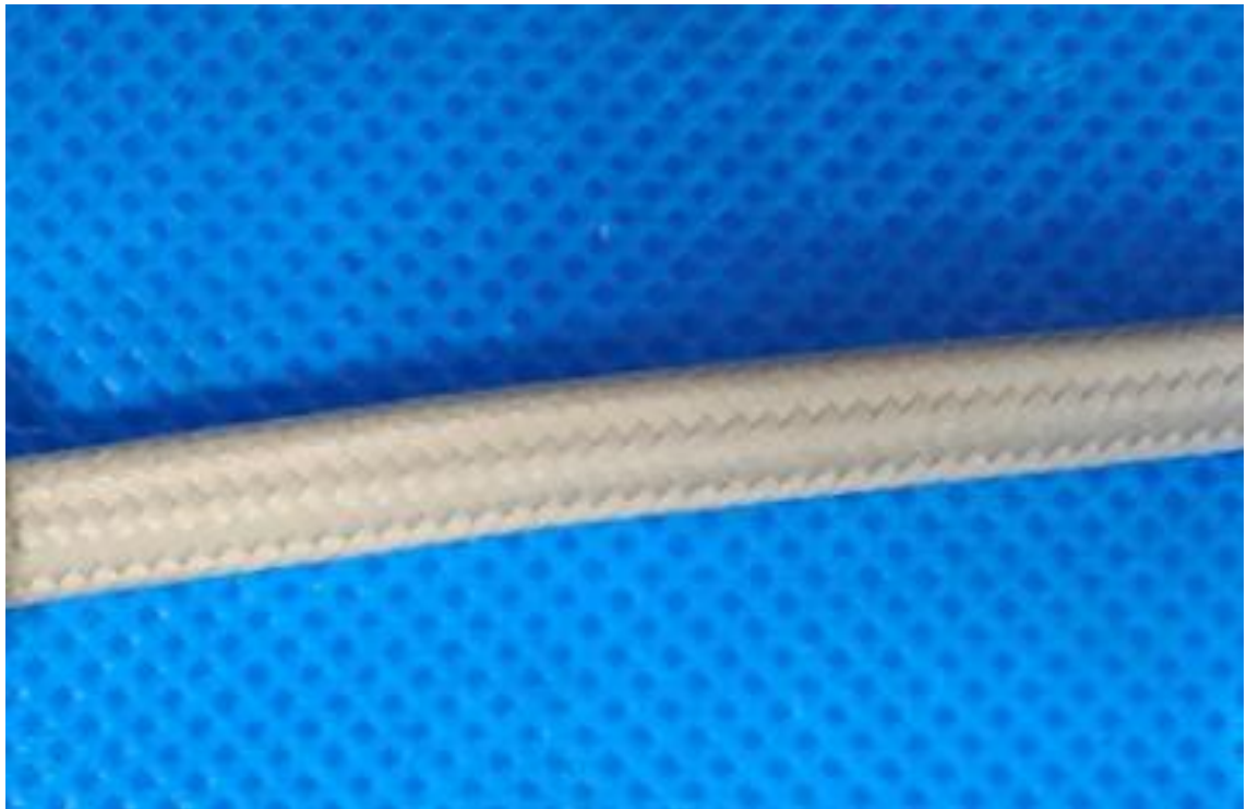
Photo 20: fibre sleeving view
