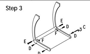
The bottom plate and legs are fixed with EDF three types of screws and tightened with C
