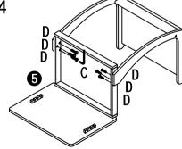
Secure the panel and bottom box with screw D and tighten with a hex wrench C
