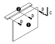
Install the bottom plate and cross bar with screw D and tighten with Allen wrench C
