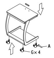
Install four G universal wheels at the bottom ( Use A wrench to install )
