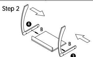
Align wood pin B with the hole in the middle of each leg and connect the bottom panel
