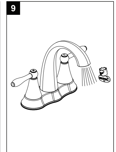
Remove aerator assembly and flush out debris. Reinstall aerator assembly.
