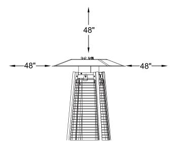
CAUTION: ANY MATERIALS OR ITEMS THAT ARE STORED ABOVE, BESIDE OR UNDER THIS HEATER WHILE IN USE WILL BE SUBJECT TO RADIANT HE AT AND COULD BE SERIOUSLY DAMAGED.
