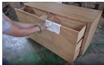
Apply a 10 lbf (44 N) horizontal force, not tip over
