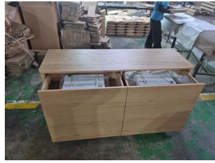
Load each drawer weighs 12kg, not tip over .
