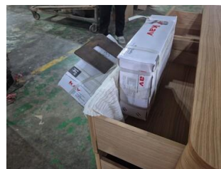
60lbs weight at the highest-level drawer
