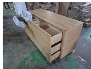
60lbs weight at the highest-level drawer
