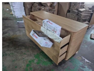
60lbs weight at the highest-level drawer
