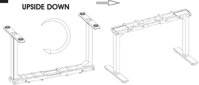
**5** Attach lifting legs, feet and pads with M6 screws as shown.
