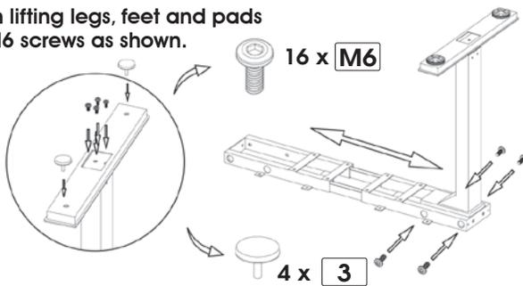
**6** Attach brackets with M6 screws as shown.
