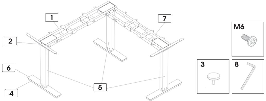
**1** Loosen all 8 screws under the structure to allow adjustment of the length.
