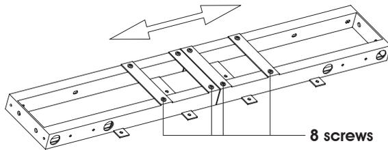
**2** Attach lifting legs with M6 screws as shown.
