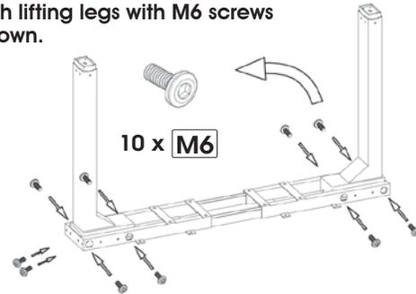
**3** Attach feet and pads with M6 screws as shown.
