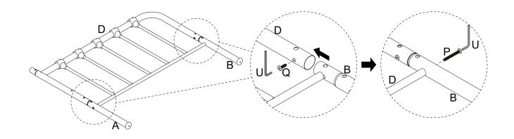
Attach Back Frame (E) to Arm (C & D) using Bolt (Q & P) with Allen Key (U).
