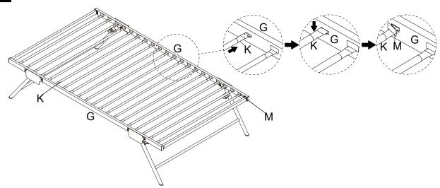
Connect Slat (K) using Slat Spacer (L) as shown.
