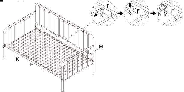
Connect Slat (K) using Slat Spacer (L) as shown.
