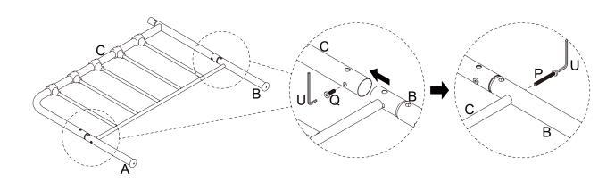
Attach Post (A & B) to RSF Arm (D) using Bolt (Q & P) with Allen Key (U).
