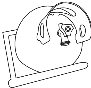
Fig. 20 Place LP tank in cradle. Lift cradle slowly until tank is upright.
