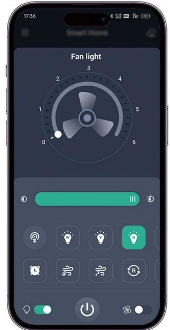
Step6 Turn on the matching button. In order to ensure that the application successfully controls the device, please click the "📶" button within 5 seconds of the device being powered on. If the device flashes or beeps, it means that the phone and the device are successfully matched, and the lamp can be controlled through the application later.
