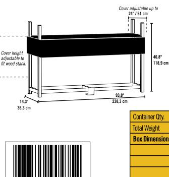
Package Includes 1 x 2 in. / 2,5 x 5,1 cm Rectangular Steel Frame 2 Way Adjustable Polyester Cover I-Beam Reinforcements Hardware Kit
