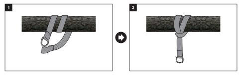
Figure 2: Connect the tree straps and ropes with carabiners.(Attention: make sure the screw lock of carabiner is 100% tightened.)
