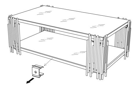
**Notes:** Remove the metal buckle after installation
