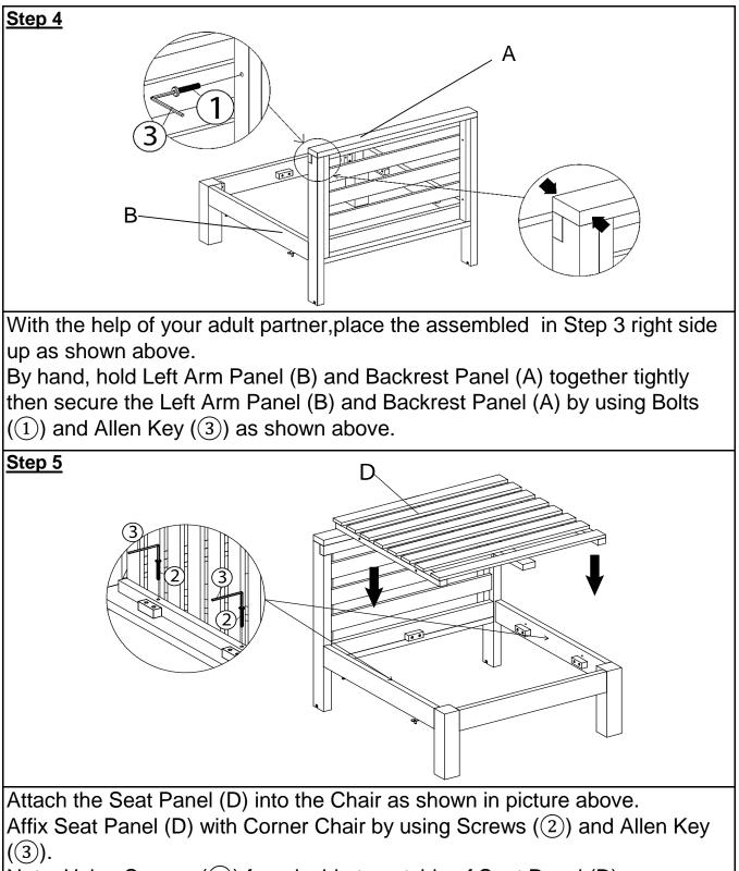
Note: Using Screws (2) from inside to outside of Seat Panel (D) **DO NOT FULLY TIGHTHEN SCREWS.**
