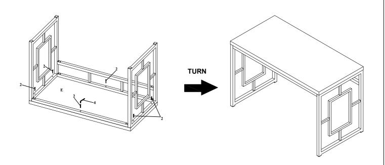
Step 2: Place Table Top (E) on a soft and clean surface to prevent finish from scratching. Place the table assembly in Step 1 onto Table Top (E) . Insert the Long Bolt (2) into the holes of LSF/RSR Leg Frame (A,B), and secure with an Allen Key (4). Fully tighten all bolts at this time.
