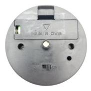
2. Turn the on/off switch to the "on" position. Replace the solar panel top and turn clockwise to lock into place.
