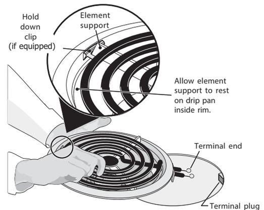
Figure 14: Removing coil and drip bowl
