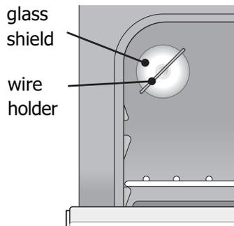
Figure 21: Oven light protected by glass shield
