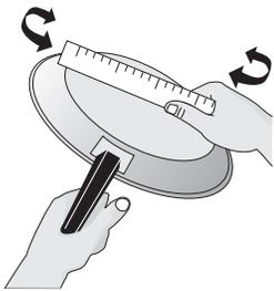
Check for flatness by rotating a ruler across the bottom of the cookware (see Figure 1). Cookware should have flat bottoms that make good contact with the entire surface of the heating element (see Figure 2).
