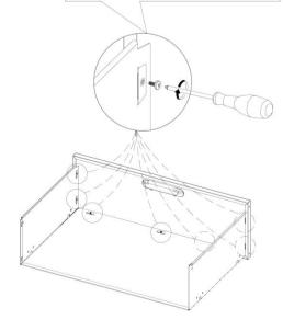
Make sure that the little bits protruding from part 12 are all inserted.
