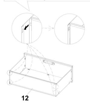
1.pill out the small rails in the slide rails on the side
