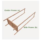
1 Position Side frame (b), Center Frame (c) and Bottom Panel (f) as picture shown. Secure them with Long Screws
