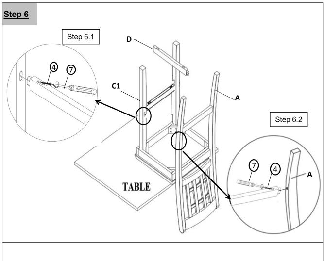
Next place Side Rail(D) into the housing of the Hind Leg of the Chair Back(A) and Left Front Leg(C1).
