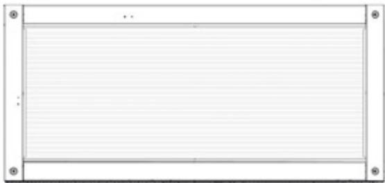
WA03 WINDOW ASSEMBLY - W2A04163 (x1) 1 7/8"x21 13/16"x47 3/16" (48x554x1198)
