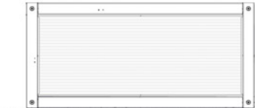
WA04 WINDOW ASSEMBLY - W2A04164 (x1) 1 7/8"x21 13/16"x47 3/16" (48x554x1198)
