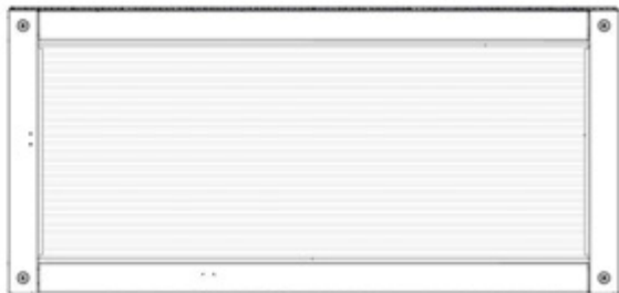
WA04 WINDOW ASSEMBLY - W2A04164 (x1) 1 7/8"x21 13/16"x47 3/16" (48x554x1198)
