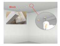
Step5 Apply glue to the second wood block: Apply glue to the interface of the second wood block and the inner part of the column. Apply a generous amount of glue to ensure a strong bond between the wood block and the ground.
