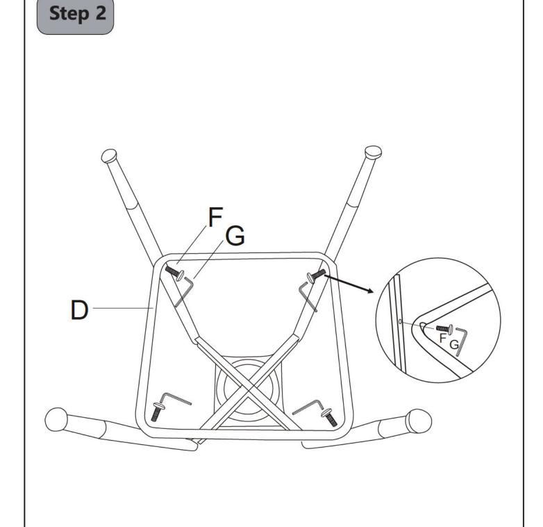
Attaching Footrest D to Legs B. Align the holes on the Footrest D with the holes on the Legs B. Secured with Screws F and Allen Wrench G. Tighten all the screws.
