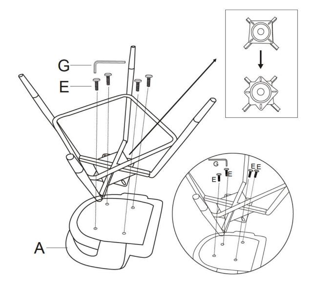
Attaching Swivel Plate C to Seat A. Align the holes on the Swivel Plate C with the holes pre-drilled on the bottom of the Seat A. Secured with Screws E and Allen Wrench G. Tighten all the screws.
