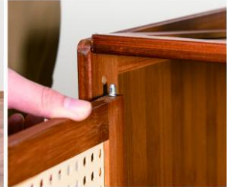
12. Install the door panel and insert the metal clip on the door panel into the hole on the ceiling panel.
