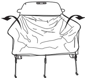
3. Attach the small hooks found at the front corners of the tent floor to the bed's tie down hooks located near the cab.
