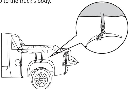
5. Locate the tent tailgate straps (3). Slide the 3 straps with the male clip between the truck box and the tailgate (you may have to lift the tailgate to do so). Connect the male clip strap to the corresponding strap with the female clip.
